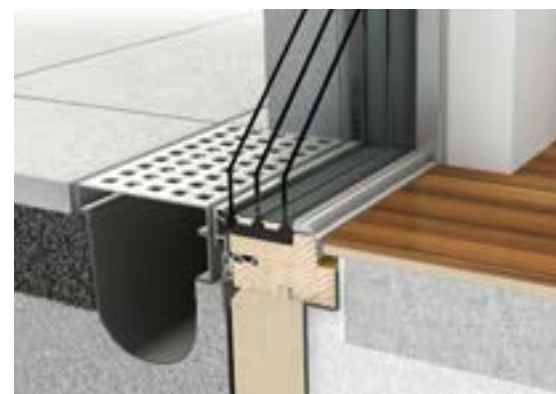
Frameless appearance and technologically optimized construction connection
